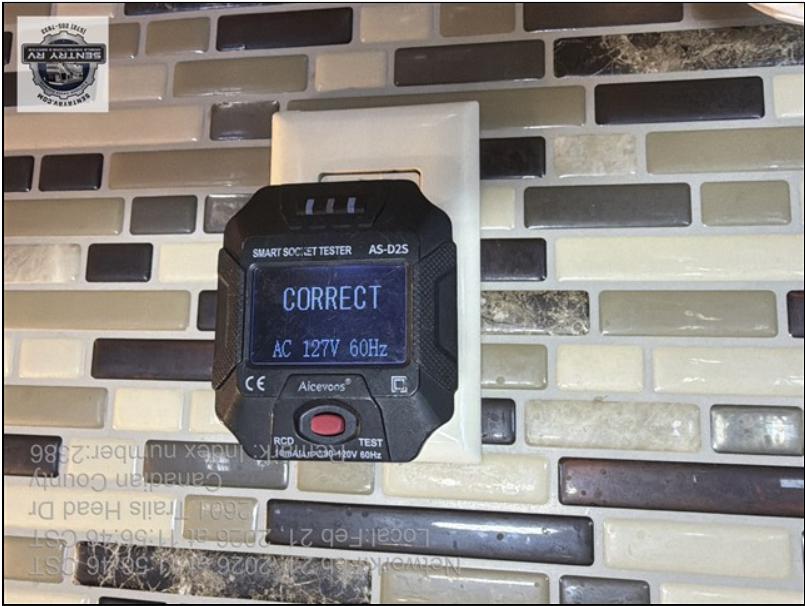
Voltage/Polarity/Frequency Test Kitchen Wall
