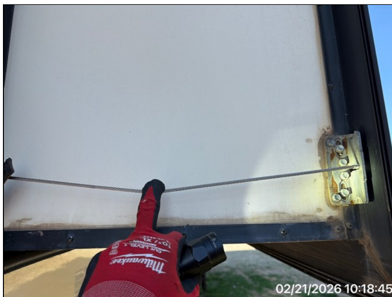
Streetside Front Slideout Cables
